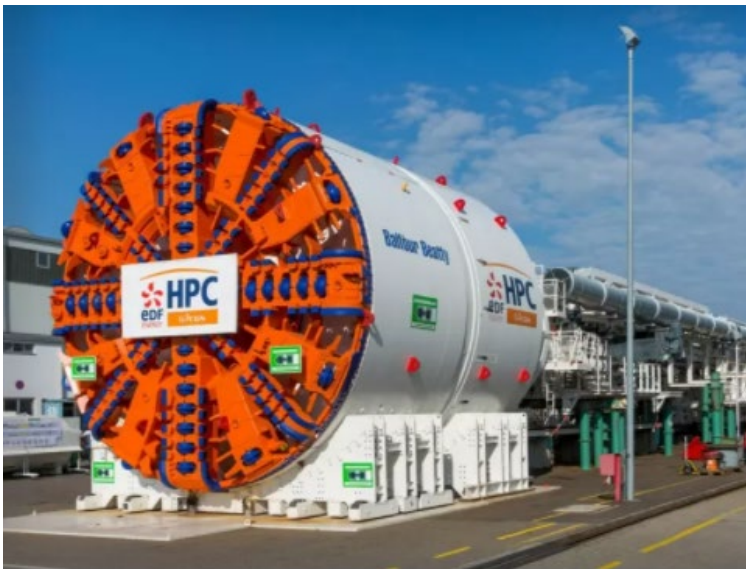
A tunnel boring machine being used at Hinckley Point C. Image: Balfour Beatty and Hinkley Point C (used with permission).
