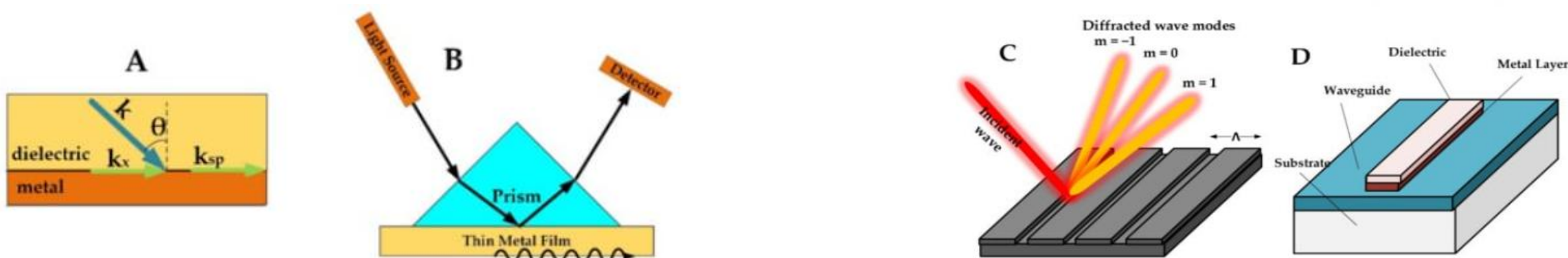
(A) Geometry for surface plasmon wave. (B) The basic Kretschmann configuration. (C) Diffraction grating configuration. (D) Waveguide configuration
