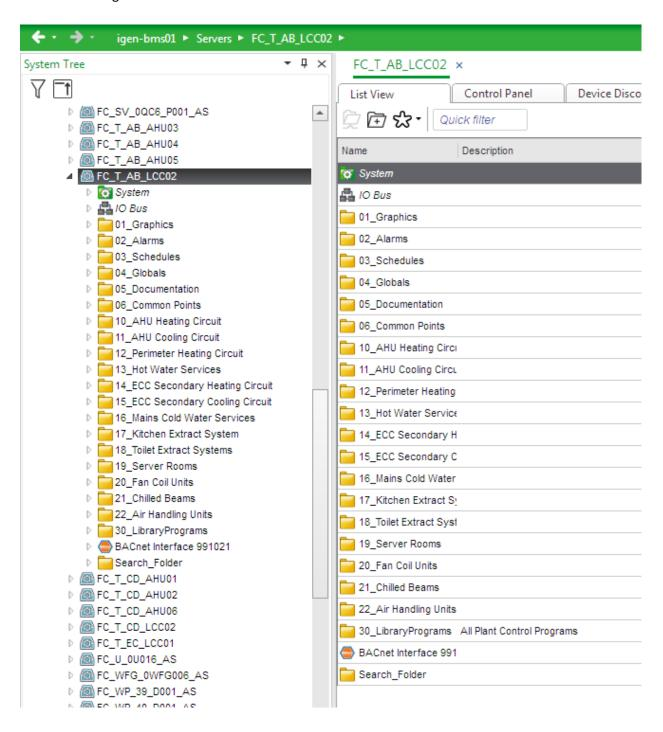
Subsequent folders and sub-folders shall be created to accommodate the plant controlled in a logical order. Examples:
