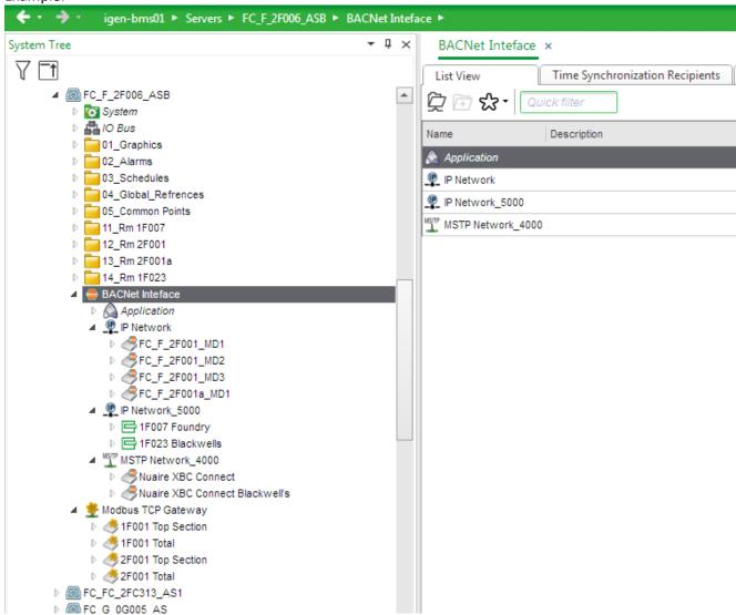
Where points from these controllers are attached to graphics (either Infinite and/or BACNet), then they shall have a duplicate point created in the Application folder, which is bound to the graphic and the controller point.
