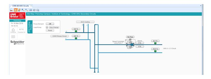
NO panels shall include Hand/Off/Auto switches or indication lamps (except panel power etc.) and therefore a graphic shall be produced to mimic how the panel fascia would have looked. The I/O module switches shall provide feedback to indicate the H/O/A status and the digital inputs shall provide condition status.
