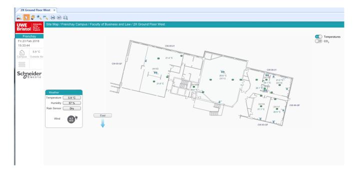
By selecting an individual room a pop out graphic displaying the room control detail and providing the operator access to override or change settings and time schedules. A "Reset Zoom" button returns to the original floor plan.
