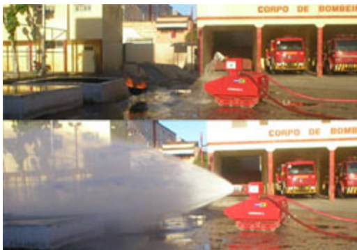
A robot equipped with a firefighting cannon. Image: Aeborah at Portuguese Wikipedia, Public domain, via Wikimedia Commons.
